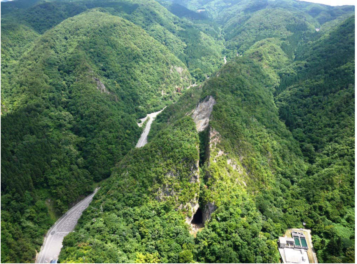
Doyu-no-warito Opencut Site (aerial photo). The crack on the summit is some 30m wide and 74m deep. It held a mother lode about 10m across called the Doyu Vein.
